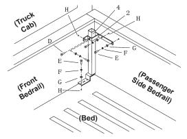
Attach the assembly to the Blind Fasteners as shown above using Bolts (E), Washers (F), and Spring Washers (G) - as shown above.
